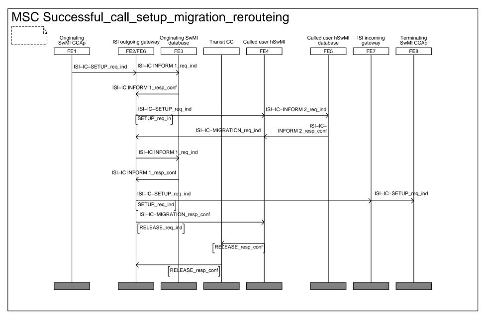
Figure 12: Information flow sequence - call set-up to a called user having migrated from SwMI B, using re-routing
