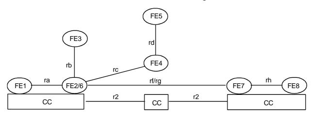
Figure 8: Example relationship between models for ANF-ISIIC and basic call in the case of re-routing
