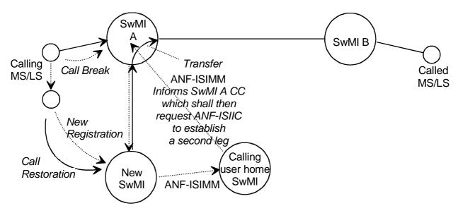
Figure 1: Call restoration by the calling user having migrated, with its home SwMI being different from SwMI A
