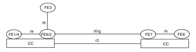
Figure 6: Example relationship between models for ANF-ISIIC and basic call in the case of called user hSwMI being SwMI A
