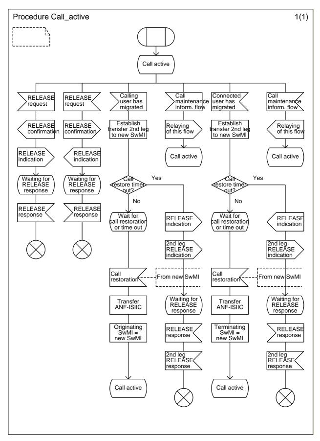
Figure 2 (sheet 4 of 5): ANF-ISIIC, overall SDL Call active procedure
