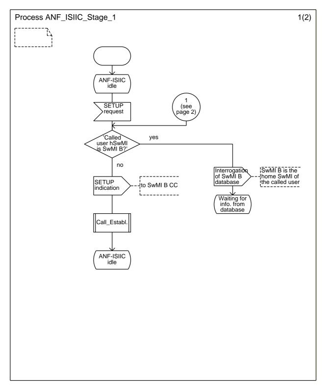
Figure 2 (sheet 1 of 5): ANF-ISIIC, overall SDL Main diagram
